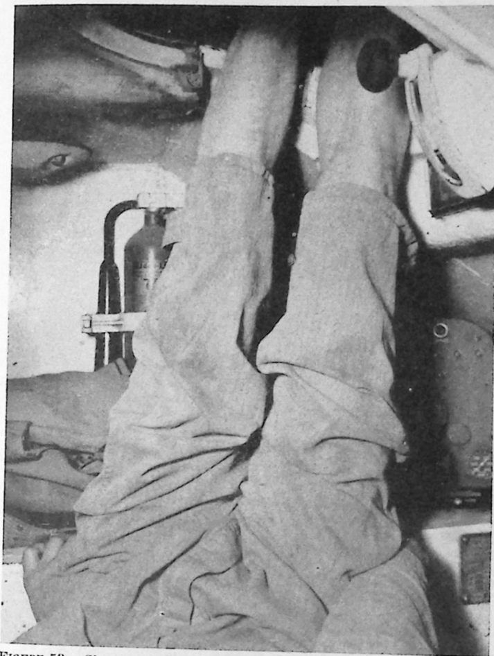
FIGURE 53.—Showing driver of M4 medium tank in position preparatory to being hoisted through hatch by the inversion method.
