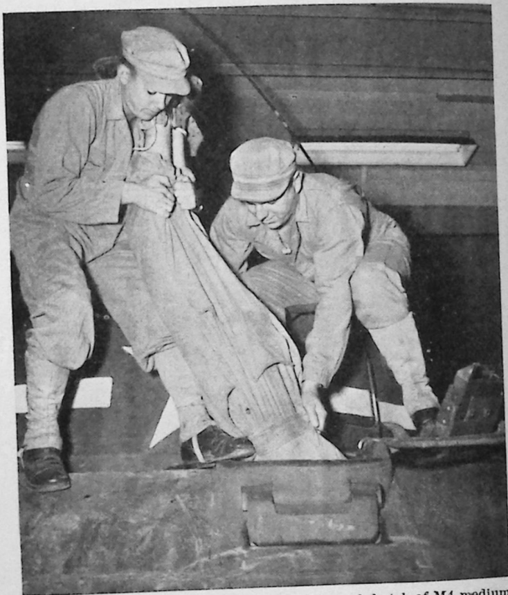
FIGURE 54.—Showing driver being hoisted through hatch of M4 medium tank by the inversion method.
